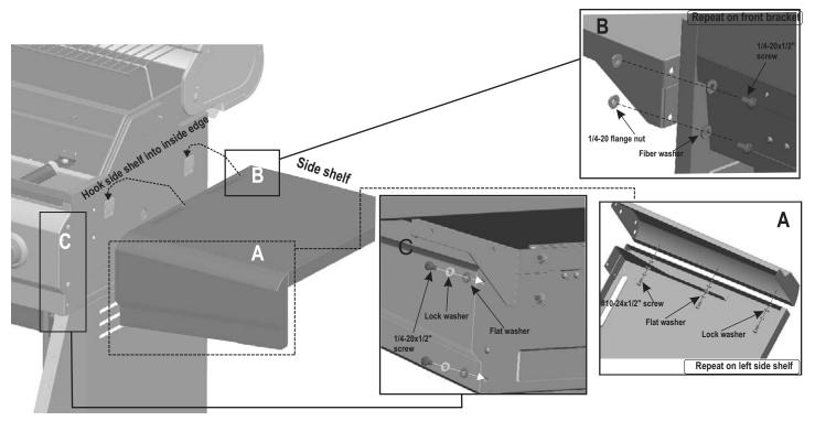
Repeat step 7 (A) on left side shelf. Hang sideburner shelf on the tabs mounted on the firebox. Attach shelf brackets to cart side panel using two 1/4-20x1/2" screws, fiber washers and 1/4-20 flange nuts on each bracket (A). Secure fascia to firebox using two 1/4-20x1/2" screws, 7mm lock washers and 7mm flat washers. Place drip pan on the sideburner shelf with four #8x3/8" self-tap screws and 5mm fiber washers (B).
